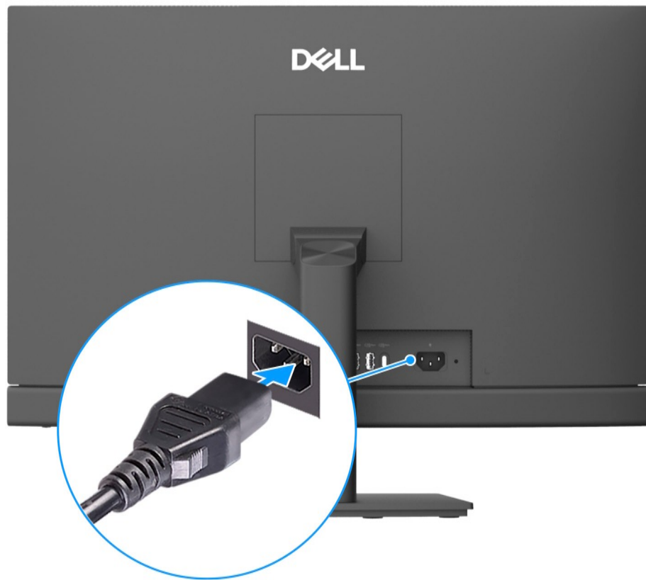
Figure 10. Connecting the power cable
